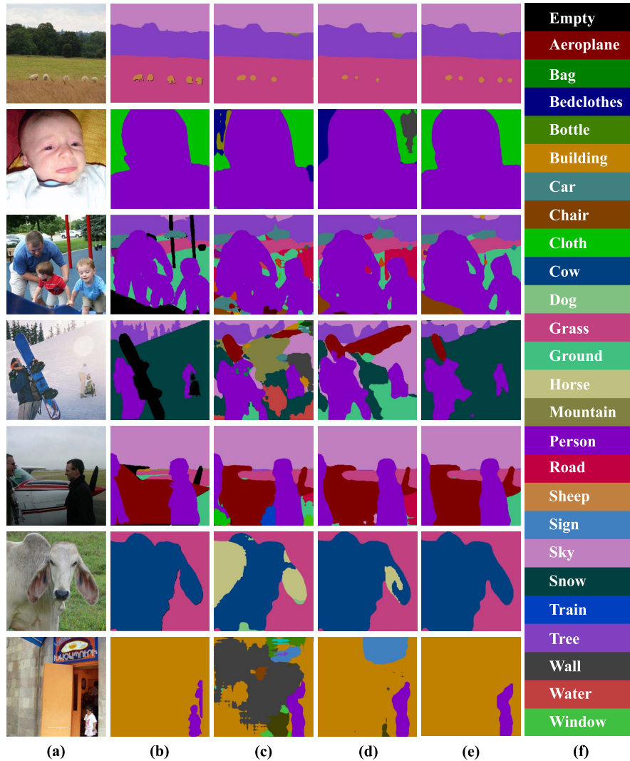
Fig. 6. Qualitative comparison with baseline Dilated FCN and Basic SA on PASCAL-Context test set. (a) Original image. (b) Ground-truth masks. (c) Results of Dilated FCN. (d) Results of Basic SA. (e) Results of our ORDNet. (f) Legend of semantic categories.
